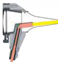
Direct Xenon Halogen illumination
