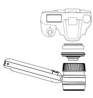
The HEINE SLR | SLM Camera Adapter flow can be used with a DSLR or DSLM camera with an existing fixed focal length lens that has an M52 or M49 connection thread. It is suitable for use with the HEINE DELTA 30 PRO and the HEINE DELTA 30. Any reference to the DELTA 30 PRO in this document is a reference to both instruments.
