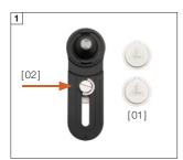
▲ Keep the fixing button [01] separate from the magnetic holder before attaching it to the phone case!
