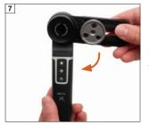
In place of the Magnifier Module, position the smartphone adapter so that it is flush, and turn it clockwise to secure it. Check that the adapter is sitting completely flat against the entire surface and is fully engaged.
