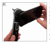
To make fine adjustments, adjust the smartphone camera with the otoscope so that a clear image is visible on the switched-on display. Tighten the screw on the adapter.
