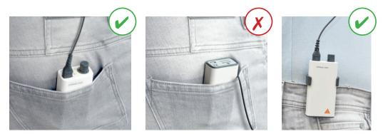
Ensure that you put your mPack mini power source with the "head up" in your pocket. Wearing the mPack mini bottom down, the cord can not be ripped out of the plug in the battery pack, thus could lead to intensive stretching and bending which leads to breaking or intensive wear & tear. For proper handling, we recommend to always use the "mPack mini belt clip" that comes along with this shipment.
