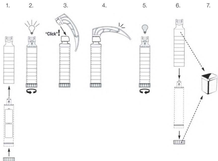
The XP disposable handle shell was especially designed for use with HEINE laryngoscope inserts. The HEINE laryngoscope insert is placed inside the disposable handle shell and the light is activated by turning the bottom insert. Following intubation, the user simply unscrews the bottom insert and the laryngoscope insert can be removed with no risk of contamination. The handle shell, the bottom insert and the XP blade are all disposed of.
