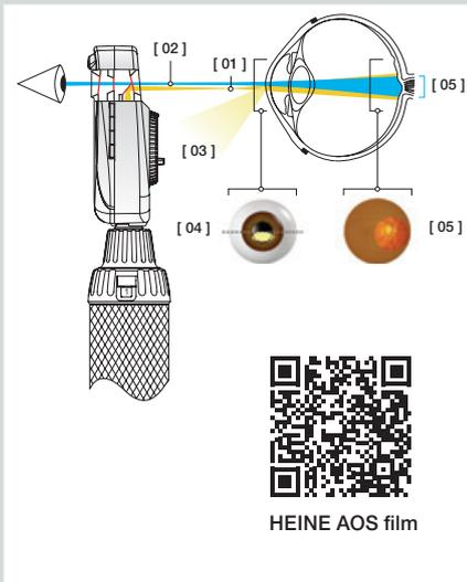
“Aspherical Optical System” (AOS) exclusively from HEINE eliminates corneal and iris reflexes to provide large, crisp and glare-free fundus images.
