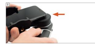
The magnet on the adapter now keeps the smartphone in position on the focusing ring of the dermatoscope.
