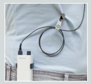
4) Always try to keep the cable close to your body or beneath your lab coat. The cable clip can help you to attach the cable as required. Also make sure to keep the cable as short as possible to avoid getting it caught on any equipment. Use the cable holder to coil up the cable. Simply roll it up 2-3 times as seen in the picture:
