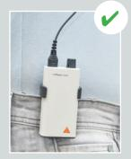
2) Ensure that you put your mPack mini Power Source with the "head up" in your pocket. Wearing the mPack mini bottom down, the cord can not be ripped out of the plug in the battery pack, thus could lead to intensive stretching and bending which leads to breaking or intensive wear & tear.
